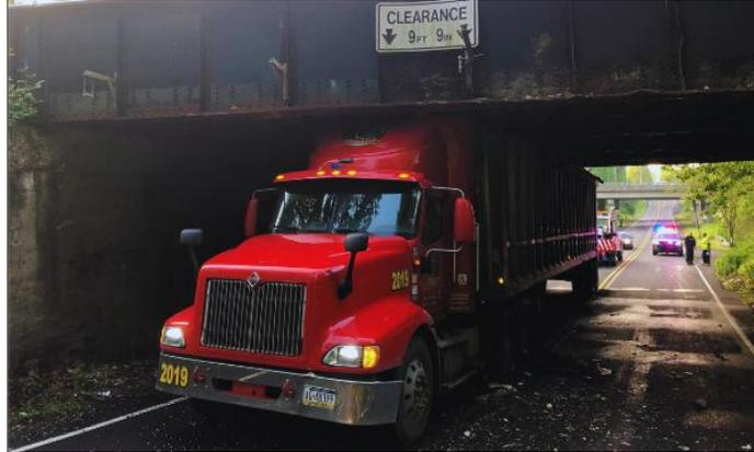
A mast arm is proposed to be repurposed to this area to provide large vehicle operators with more advanced notice. A study to identify a solution in this area is proposed in future years. This study would recommend the best method to prevent trucks from getting stuck.
